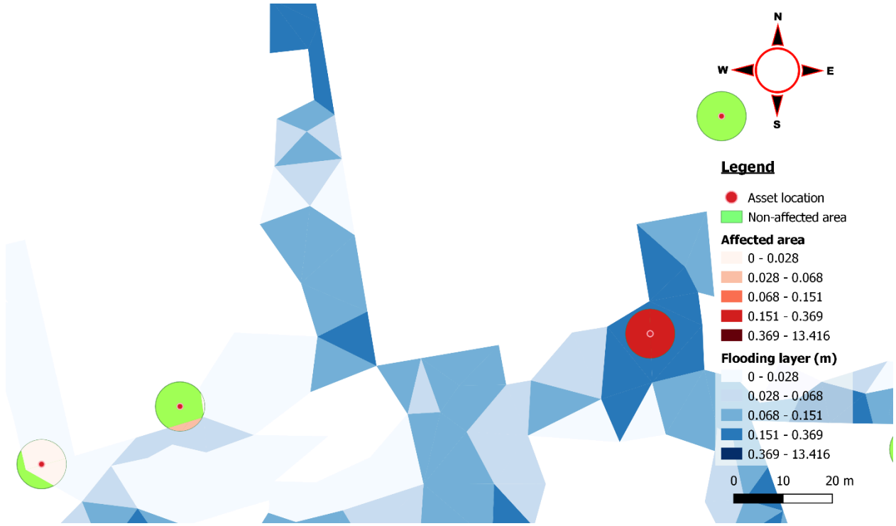
Figure 6. The sampling method based on measuring the affected and non-affected areas and the water depth data contained.
